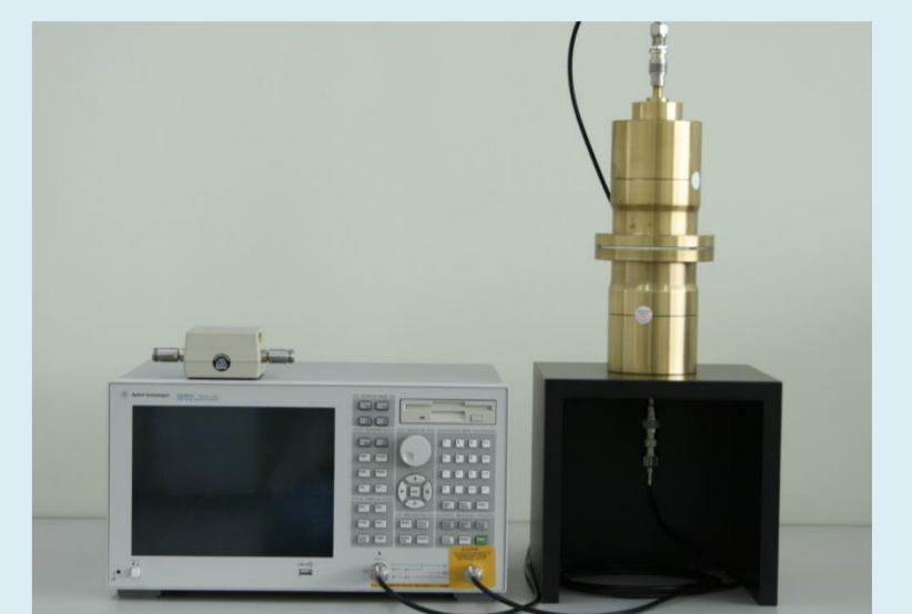
Shielding Effectiveness measurement using ASTM D4935 test fixture
