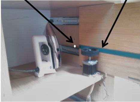
Heat source: Iron box with wooden shutter
