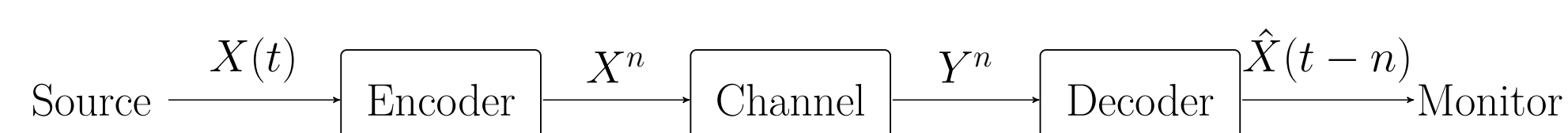
Figure 1: We show an abstract discrete time communication model for a source with m -bit information X(t) at time t .
